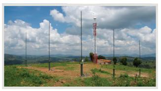
> For direction finding and signal acquisition, the system is typically configured with a nine-element Model 632 monopole antenna array. Optional TCI and third-party antenna arrays also are compatible.
