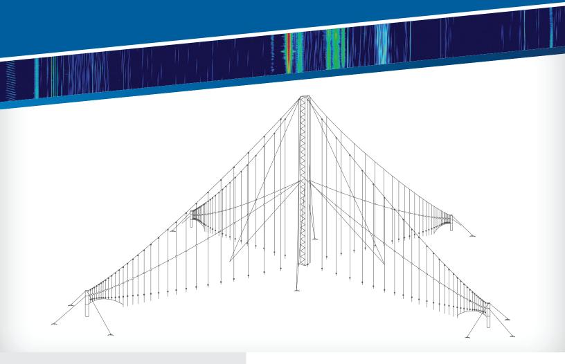
The Model 504 family of rosette dipole log-periodic antennas is designed to provide high gain, high front-to-back ratio, steerable performance in a compact area. The 504 finds wide application for ground-air and shore-ship circuits, where the other end of the path is mobile, and good long-distance coverage and gain are needed.
