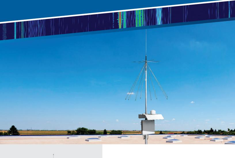
The TCI Model 640-DSC VHF/UHF antenna is designed for monitoring-only spectrum applications where direction finding is not required. The antenna provides a uniform pattern across the entire monitoring frequency band between 20 and 3000 MHz. The antenna is made of proven materials to ensure long-term operations in harsh environments.
